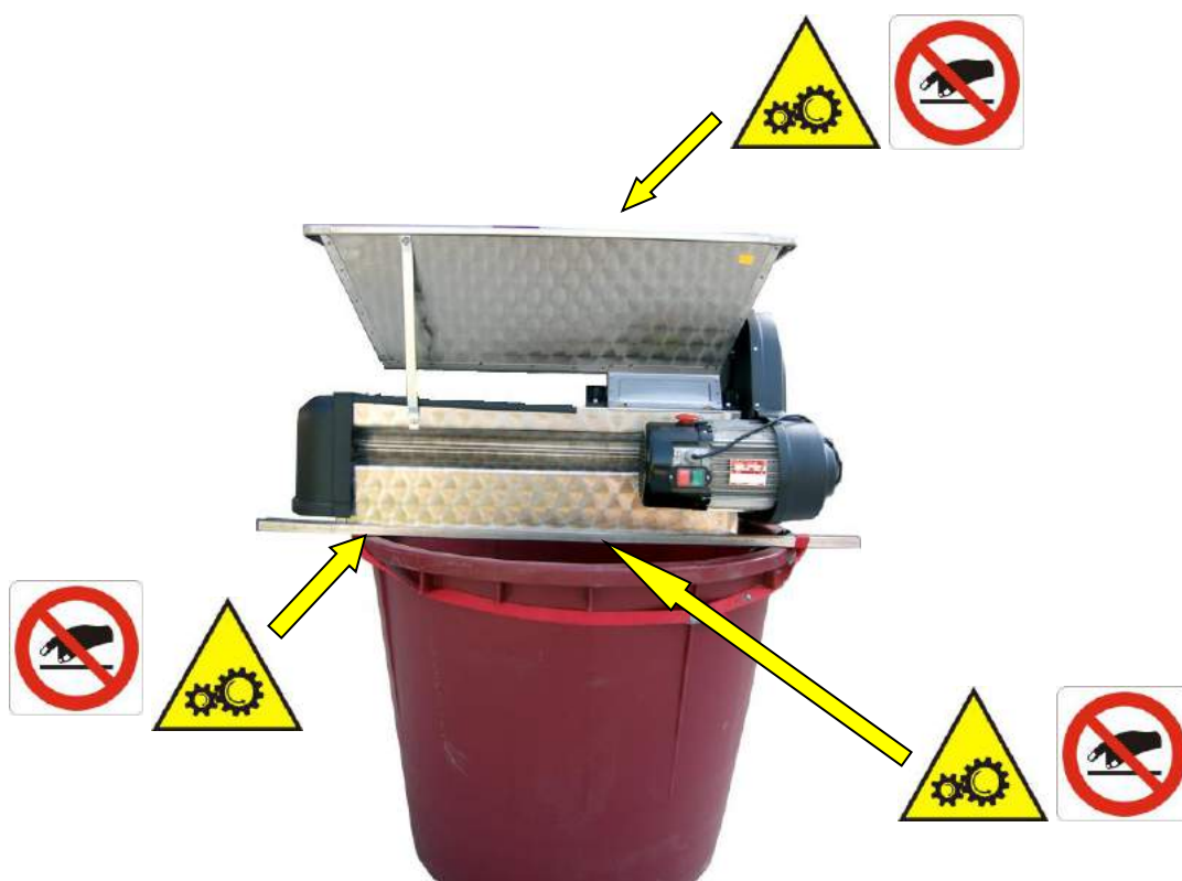
Fig. 2 Hazardous moving parts
