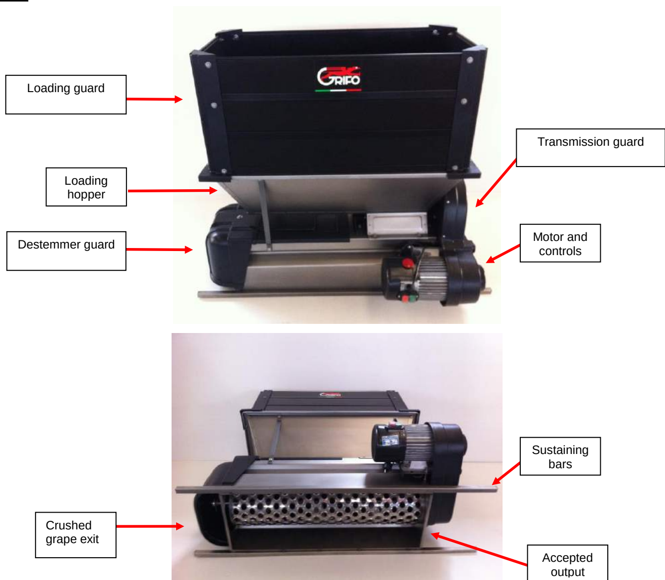
Fig. 1 Main parts of the MOTORIZED GRAPE CRUSHER AND DESTEMMER
